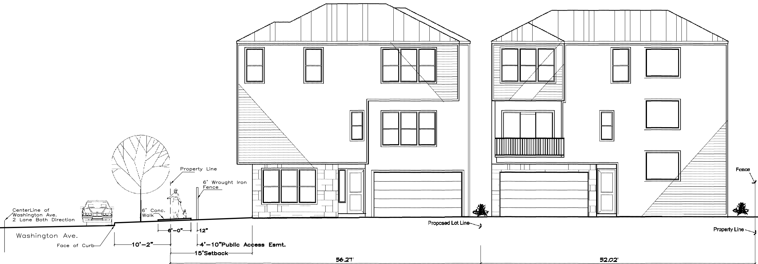
STREET DEVELOPMENT SECTIONAL ELEVATION 'C' at Center of Shared Drive Looking East 0 1 3 5 10 20'
